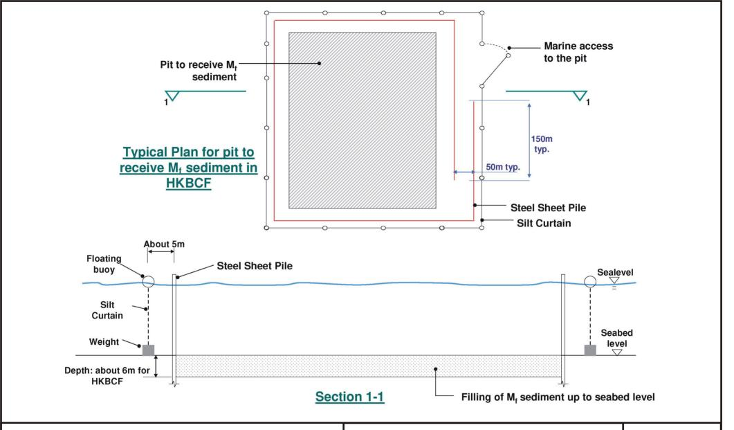
Figure 10 - Details of Silt Curtains and Steel Sheet Pile Wall 圖 10 - 防沙幕及鋼板樁牆詳情
